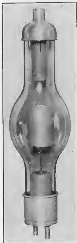
FIG. 85. A two-electrode, high-vacuum tube designed for high-voltage rectifier service.
